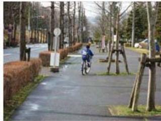
Combined (shared) off-road facilities for NMT (bicycles sharing with pedestrians) Izumi Park Town, Japan
